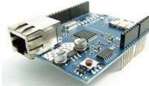
Figura 2: Tarjeta Ethernet Shield.
